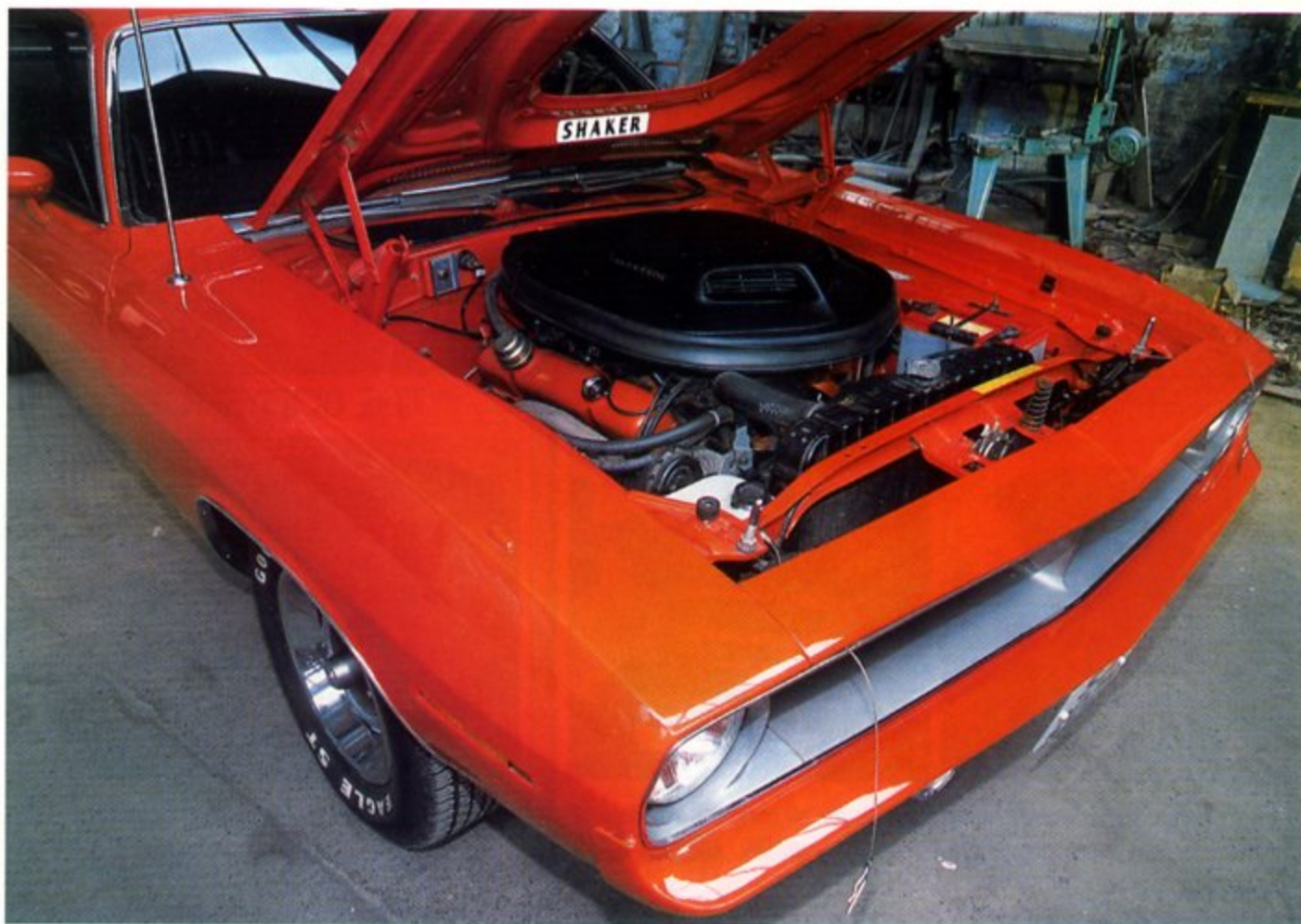
ABOVE: HIDING UNDERNEATH THAT BIG 'SHAKER' HOOD SCOOP ARE THREE TWO-BARREL CARBURETTORS. GENTLE CRUISING AROUND TOWN USES ONLY THE CENTRE CARBURETTOR, BUT WHEN THE PEDAL TOUCHES THE METAL, ALL THE CARBS OPEN UP TO ALLOW LOTS OF FRESH, COLD AIR AND BUCKET-LOADS OF FUEL IN. CONTEMPORARY ROAD-TESTERS COULD MAKE A 440-6 PERFORM NEARLY AS WELL AS A HEMI ON THE STRIP
