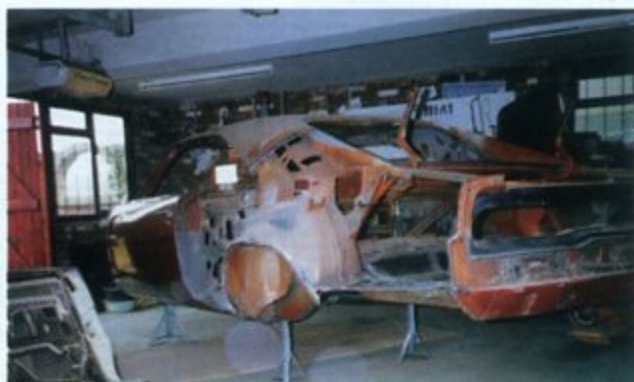
ABOVE: HEMI-CHARGER'S SERIOUS RENOVATION INCLUDED TWO COMPLETE NEW REAR QUARTERS
